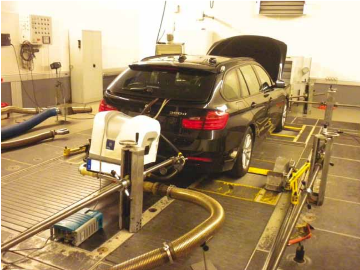
Validation of the PEMS on the chassis dynamometer
