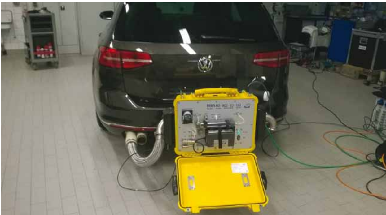
Installation of a PEMS in a car
