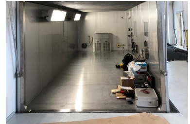
Construction of a sealed housing for evaporative determination (SHED)
