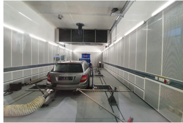
Standardized driving cycles are performed under reproducible boundary conditions (air temperature, driving profile, loads)
