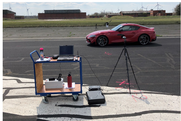
Noise emission test (Source: KBA as of April 2021)
