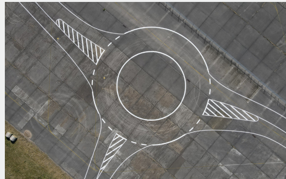
Road marking of roundabout to test critical driving situations in urban environments (Source: KBA)
