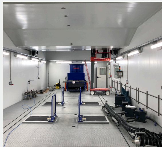
Climate roller dynamometer for different test scenarios (Source: KBA)
