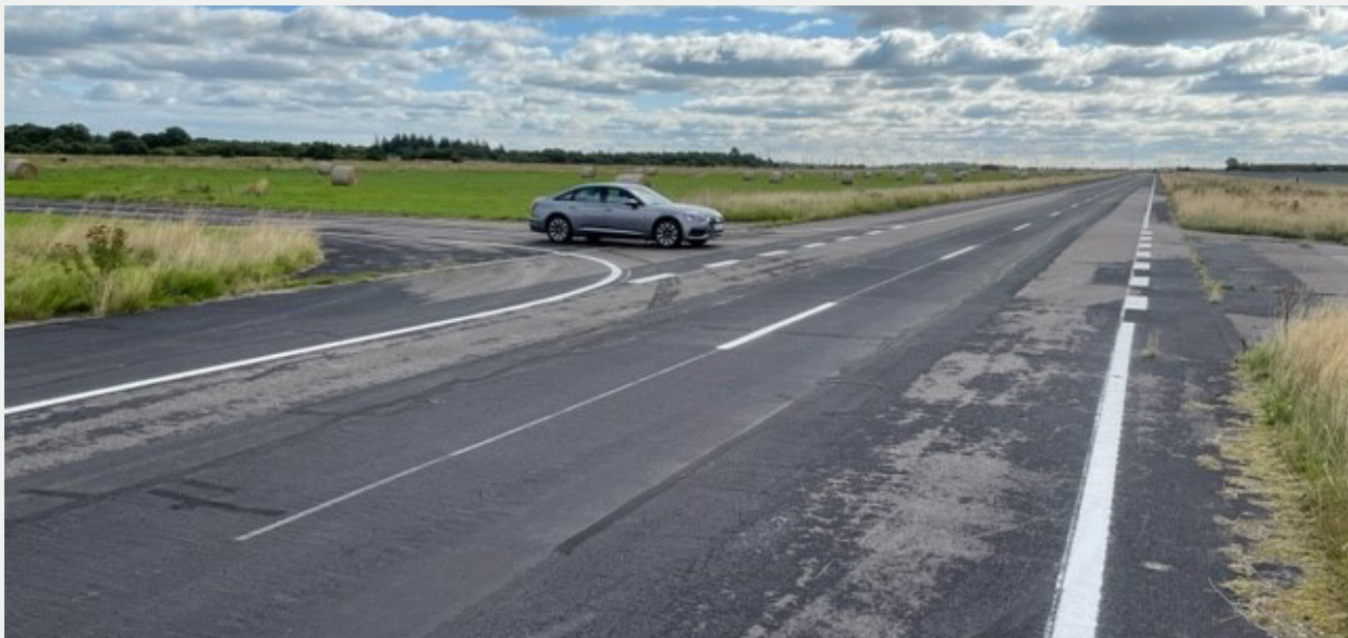
Road marking of an expressway slip for the purpose of testing vehicle behaviour in turning scenarios and on rural roads (Source: KBA)
