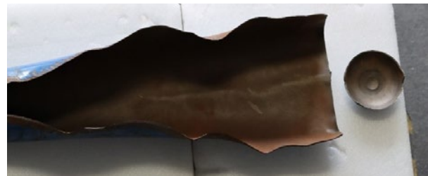
Parts of a burst gas pressure vessel
